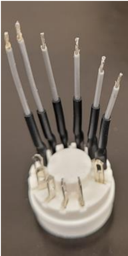
Completed PMT base with six added wires
